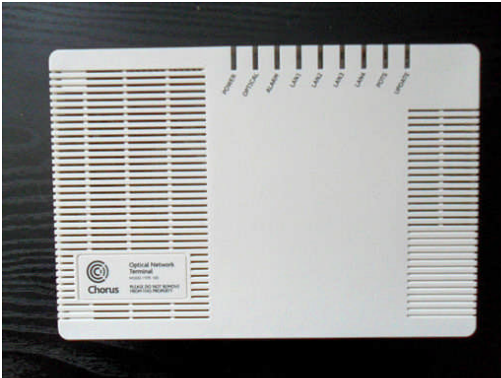
Photo 4: Optical Network Terminal (ONT) unit
